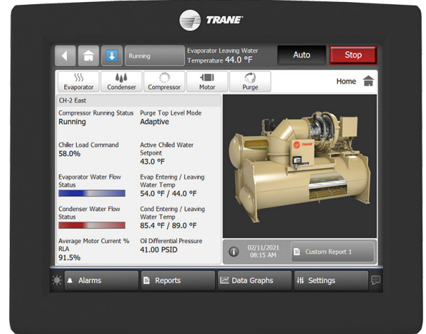
Trane customers directed the design of the AdaptiView user interface, which provides a practical approach to chiller management.
